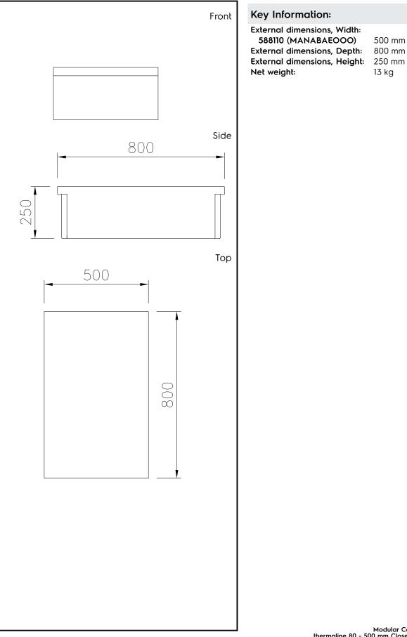
Modular Cooking Range Line thermaline 80 - 500 mm Closed Work top, 1 Side
